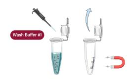
Repeat wash with 600µl of Wash Buffer #2, return to magnetic rack for 1-2 mins, then discard supernatant and leave to dry for 1 min.
